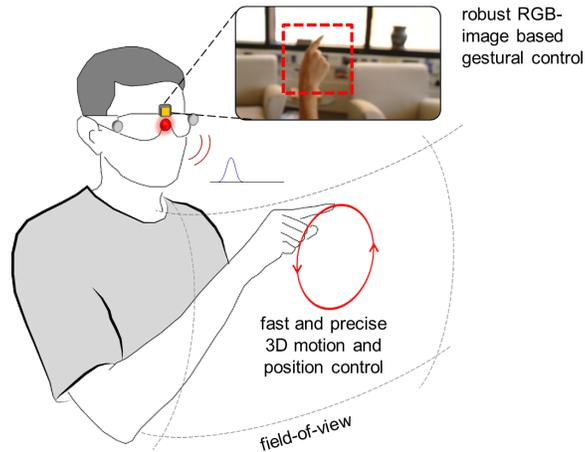
Figure 5-1: Mime combines a new TOF sensor for precise 3D tracking with RGB-image based gesture recognition.
