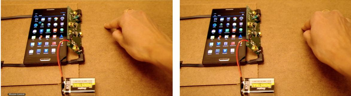
Figure 7-13: Capturing hand movements on the side of a smart phone transforms the surface immediately next to the device into a larger input space.
