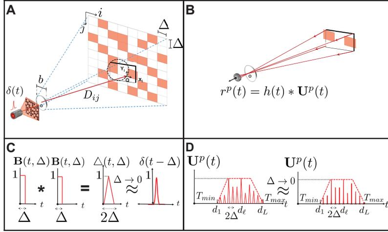
Figure 3-5: (A) Binary patterned scene illumination. (B) Scene response to all-ones scene illumination. (C) Diagrammatic explanation of the high-resolution SLM (small  $\Delta$ ) approximation. (D) Modeling of the parametric signal  $\mathbf{U}^p(t)$  as a weighted sum of equally-spaced Diracs. Note that  $\mathbf{U}^p(t)$  has the same time envelope as the signal  $\mathbf{P}(t, T_0, T_\phi \Delta\phi, T_\theta \Delta\theta)$ .
