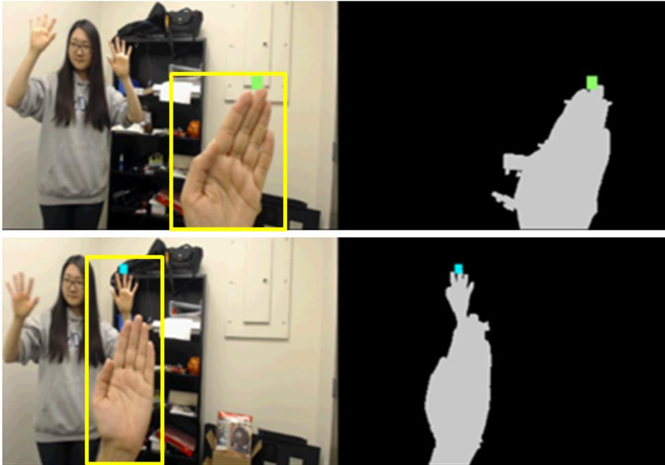
Figure 5-14: The Mime sensor's 3D localization data improves the robustness of RGB-image based gesture recognition. (Top) Notice that the skin colored targets (human hands) in the RGB camera's FOV are rejected because they do not fall inside the identified 2D ROI. (Bottom) Mime's algorithmic framework cannot be used to reject cases in which there are multiple skin-colored objects in the identified RGB ROI.
