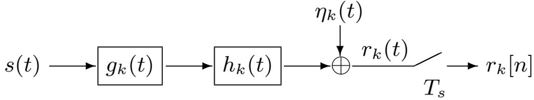
Figure 6-3: Signal flow diagram for signal acquisition at Sensor  $k$ .
