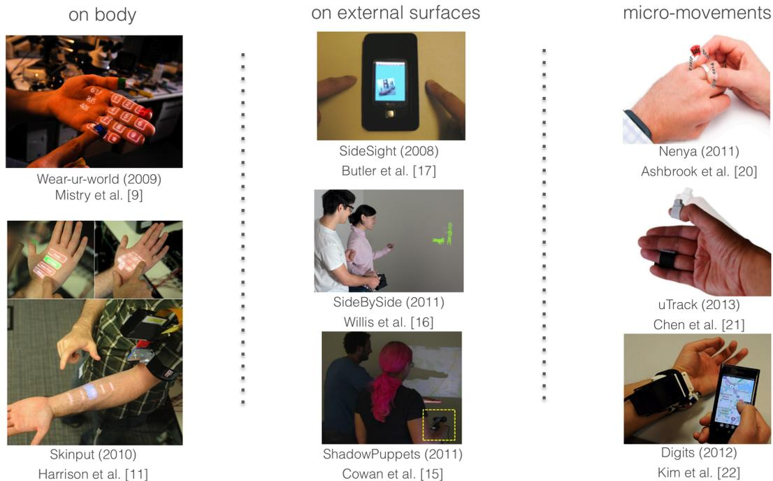
Figure 1-1: Categories of around-device interaction. On and close-to body interactions that use the body surface for a combination of input and visual feedback (left). On external surface interaction which uses surfaces like table-tops and walls around the device (middle). Micro-movements that off-load interaction without requiring much visual distraction (right).
