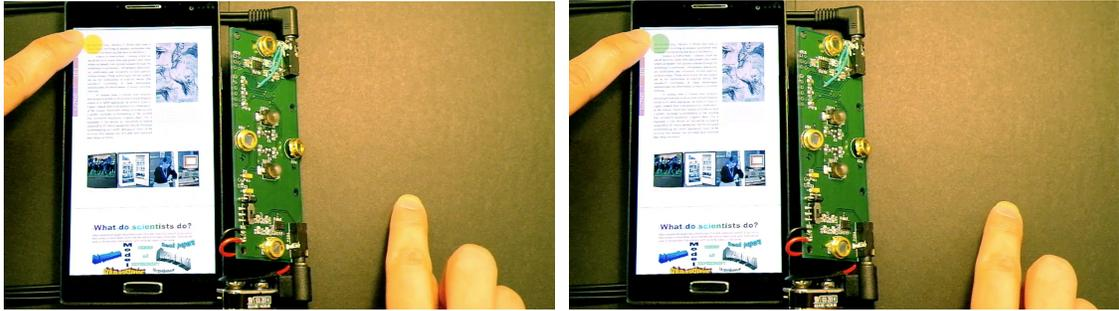
Figure 7-17: Two-handed input with touch used to select a function and side movement of the hand used to precisely control color.
