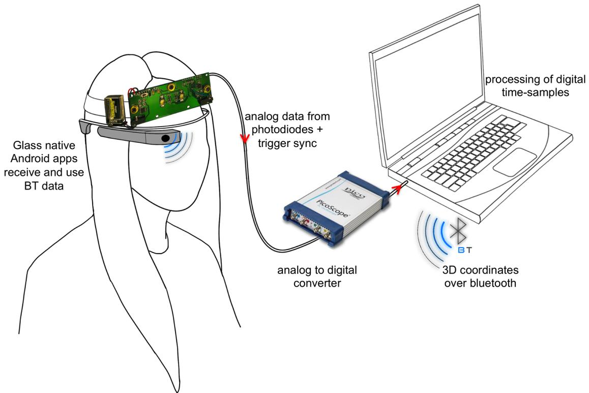
Figure 7-6: System design and data processing flow. Analog data from the sensor are received by a USB oscilloscope which transfers time samples to a laptop computer. The time samples are processed and 3D coordinates are communicated over Bluetooth to the Glass.
