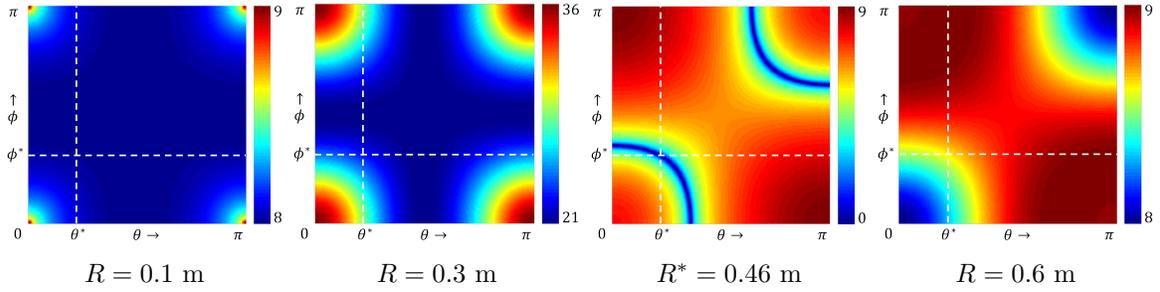
Figure 5-7: Slices of the 3D likelihood function for four values of radial distance  $R$  when the true value is  $R^* = 0.46$  m. Parameters from the hardware prototype are used: illumination by a Gaussian pulse with duration 200 ns, baseline  $2L = 10$  cm,  $T_s = 30$  ns,  $T = 100$   $\mu$ s, and  $SNR = 20$  dB.
