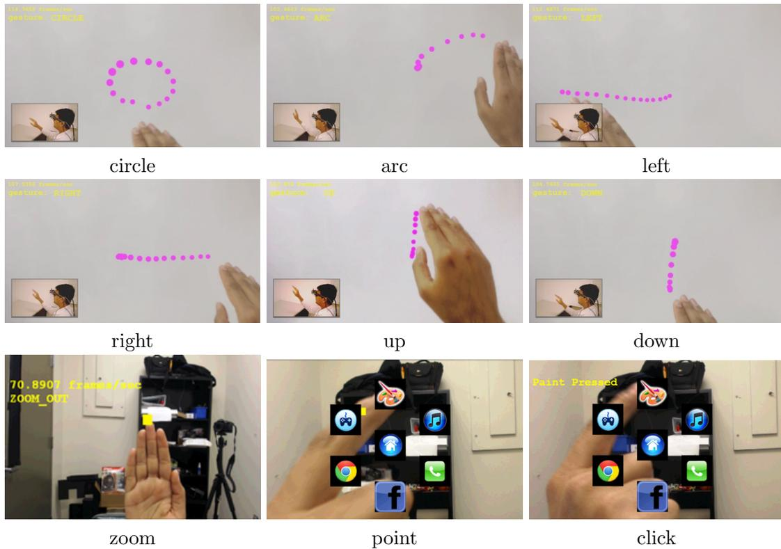
Figure 5-13: Implementation of 3D motion-activated gestures using only the 3D hand coordinates. Mime’s motion tracking works accurately in cluttered environments.
