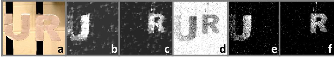
Figure 4-5: Reconstruction results. (a) Scene setup. (b), (c), and (d) Depth masks  $\mathbf{I}^1$  and  $\mathbf{I}^2$  and the background mask  $\mathbf{I}^0$  reconstructed using 500 patterns. (e) and (f) Depth masks reconstructed using 2000 patterns.
