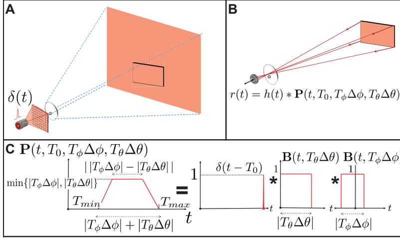
Figure 3-3: (A) All-ones scene illumination. (B) Scene response to all-ones scene illumination. (C) Diagrammatic explanation of the modeling of the parametric signal  $p(t)$ .
