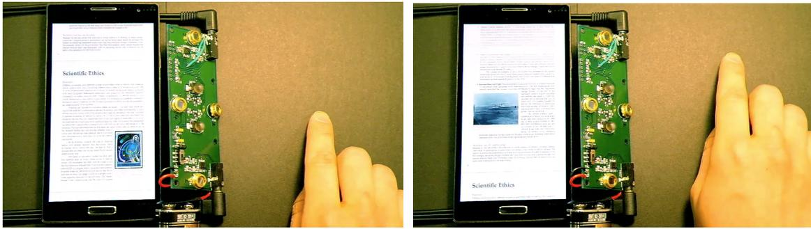
Figure 7-15: Scrolling a document by moving the hand vertically.
