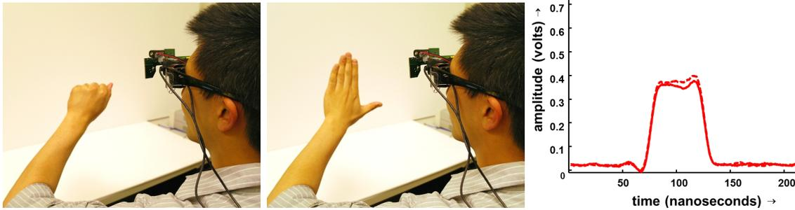
Figure 5-9: Radial fall-off dominates signal amplitude. The responses detected at a photodiode for a fixed hand position and varying hand gestures are very similar. This enables Mime to achieve robust 3D hand localization for different skin colors and gesture shapes.
