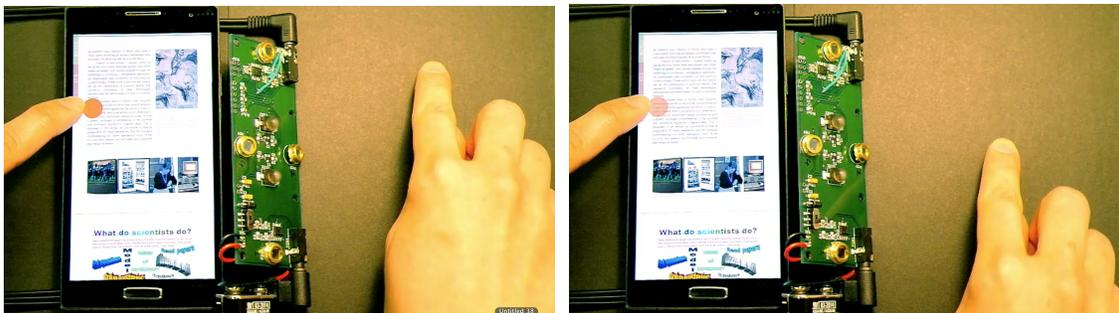
Figure 7-19: Opacity decreased by moving the hand vertically downward.
