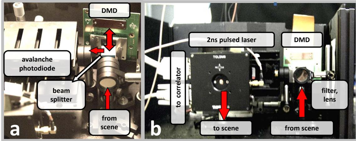
Figure 4-2: Experimental setup for compressive depth acquisition. (a) Close-up of the sensing unit showing the optical path of light reflected from the scene. (b) The complete imaging setup showing the pulsed source and the sensing unit.
