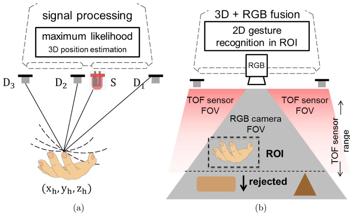
Figure 5-3: The signal processing pipeline for Mime. (a). The scene is illuminated using a pulsed LED and the backscattered light is time-sampled using 3 photodiodes. The time samples are processed using a maximum likelihood estimation framework to acquire 3D hand coordinates. (b) These coordinates are further used to identify a region-of-interest in the RGB image, and process it to recognize hand gestures.
