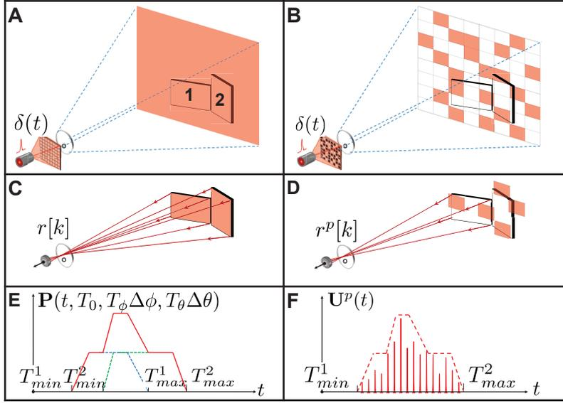
Figure 3-8: Parametric modeling in scenes with multiple planar facets. Since light transport is linear and assuming light adds linearly at the detector, the parametric signal that characterizes the scene response is the sum of multiple parametric signals. Thus even in the case of multiple planar facets, a piecewise-linear fit to the observed data allows us to reliably estimate the scene’s depth range.
