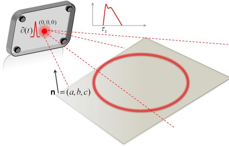
Figure 6-2: Device and scene setup for imaging single plane.
