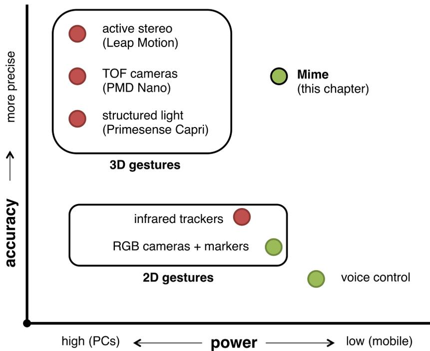
Figure 5-4: Accuracy vs. power comparison for compact, real-time HMD input technologies. The red dots denote devices with high daylight sensitivity, and green dots denote devices that operate under strong ambient light.
