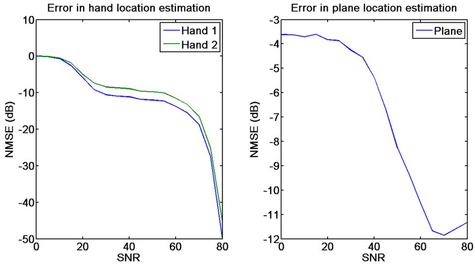
Figure 6-6: Effects of noise on scene feature estimation for (a) two fronto-parallel “hands”; and (b) a single large tilted plane.
