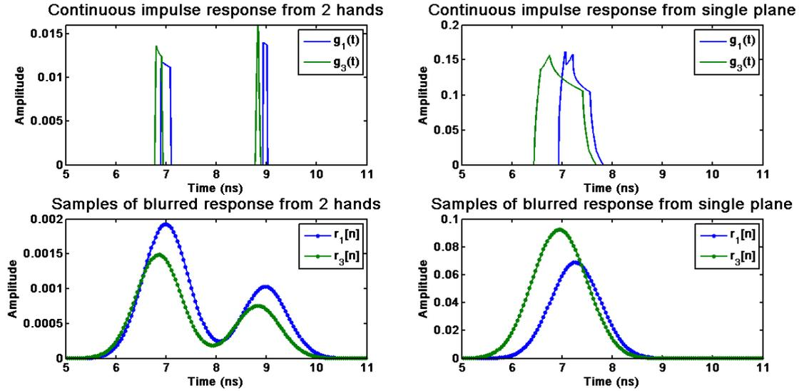
Figure 6-4: Typical continuous-time scene impulse responses  $g_k(t)$  and samples  $r_k[n]$  for our two types of scenes.
