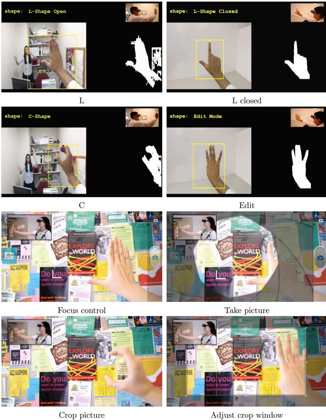
Figure 7-4: Interactive photography application with shape-based gestures implemented using Mime's 3D and RGB data fusion approach. All gestures work accurately even in cluttered environments with competing targets.
