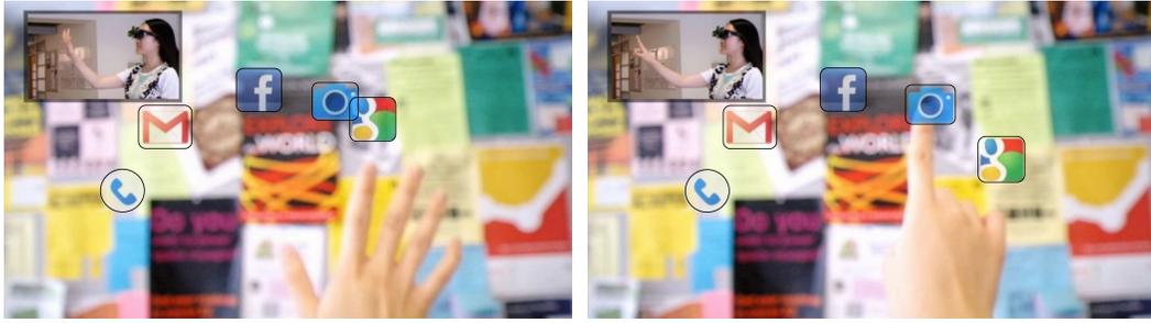
Figure 7-1: Augmented menu interaction using motion gestures: arc to activate menu, and point-and-click to select item.
