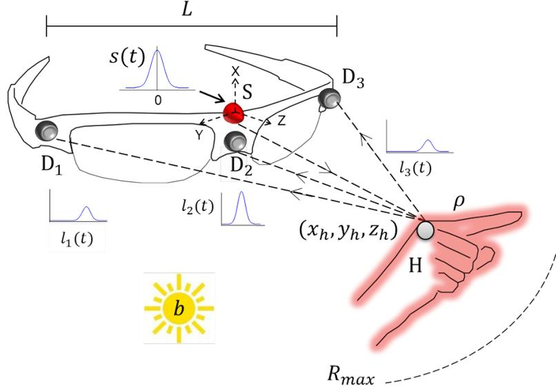
Figure 5-6: The Mime TOF sensing setup indicating the system variables and the geometric arrangements.
