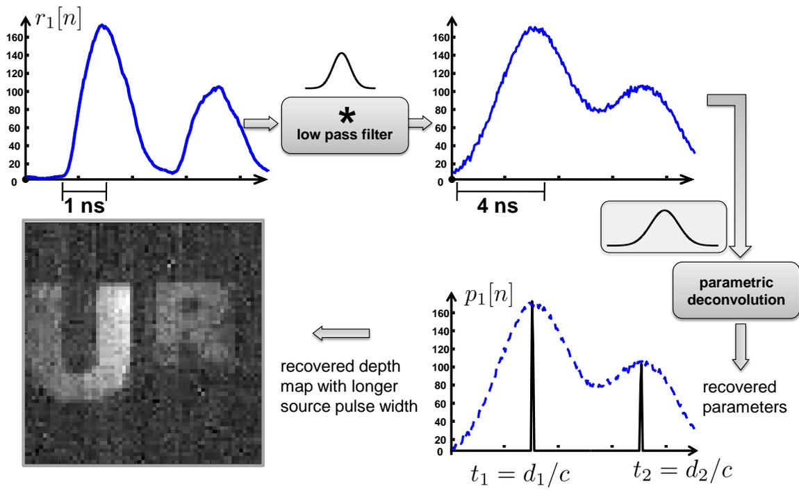
Figure 4-7: Depth map reconstruction with simulated scene response to longer source pulse width. We simulate poor temporal resolution by lowpass filtering the captured intensity profiles so that the Gaussian pulses overlap and interfere with the signal amplitudes. The effectiveness of the parametric deconvolution technique is demonstrated by accurate recovery of the depth map.
