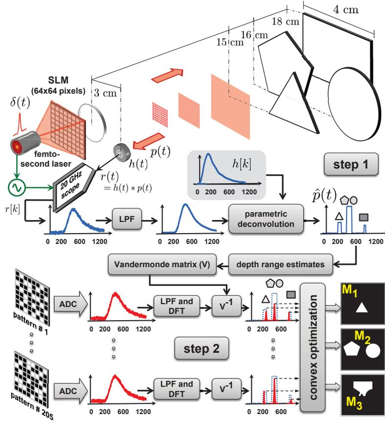
Figure 3-9: Schematic experimental setup to demonstrate depth estimation using our proposed framework. See text for details.
