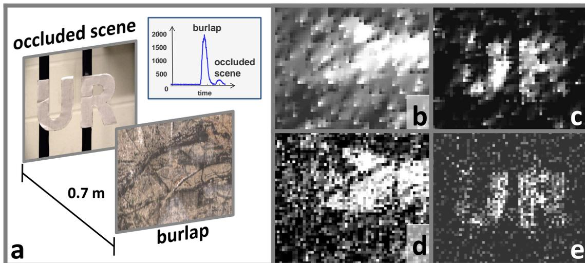
Figure 4-6: Occluded scene imaging. (a) Setup for the scene occluded with a partially-transmissive burlap; the shapes U and R are at the same depth. (b) and (c) Reconstructed depth masks for burlap and scene using 500 patterns; (d) and (e) using 2000 patterns. Note that no prior knowledge about the occluder was required for these reconstructions.
