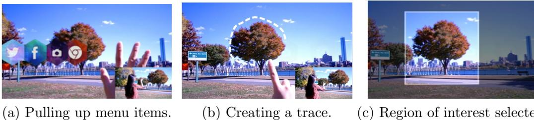
Figure 7-7: **Live Trace:** This scenario shows a user creating a trace on-the-go. The region of interest is cropped once the trace is made.
