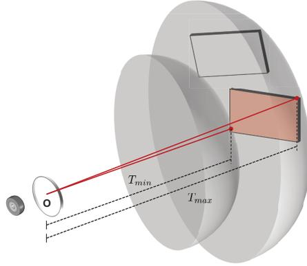
Figure 3-4: The signal  $p(t)$  only provides information regarding the depth ranges present in the scene. It does not allow us to estimate the position and shape of the planar facet in the FOV of the imaging system. At best, the facet can be localized to lie between spherical shells specified by  $T_{\min}$  and  $T_{\max}$ . In this figure two possible positions for the rectangular facet are shown.
