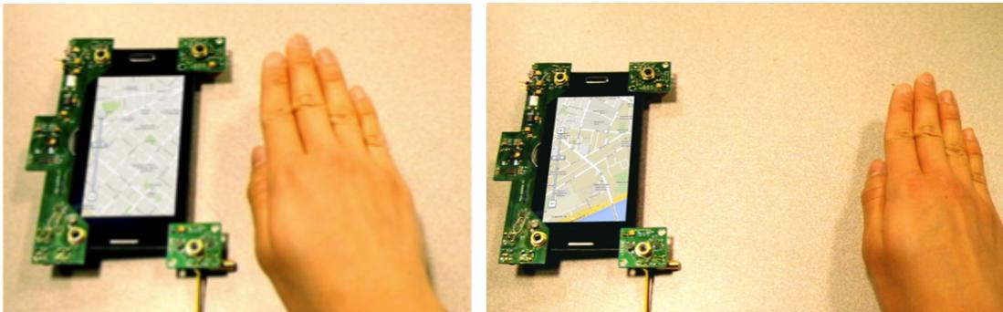
Figure 7-14: Mobile application scenario with Mime: User navigates within a map by moving their hand left to right.
