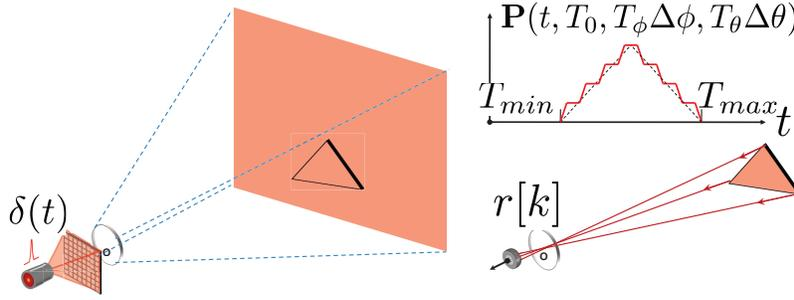
Figure 3-7: Parametric modeling for non-rectangular planes. The piecewise linear fit (shown in dotted black) is a good fit to the true parametric scene response from a triangular planar facet. This fit allows us to robustly estimate  $T_{\min}$  and  $T_{\max}$ .
