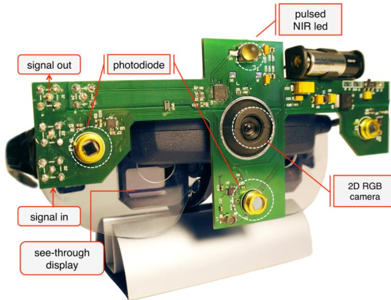
Figure 5-2: The battery powered Mime sensor prototype.
