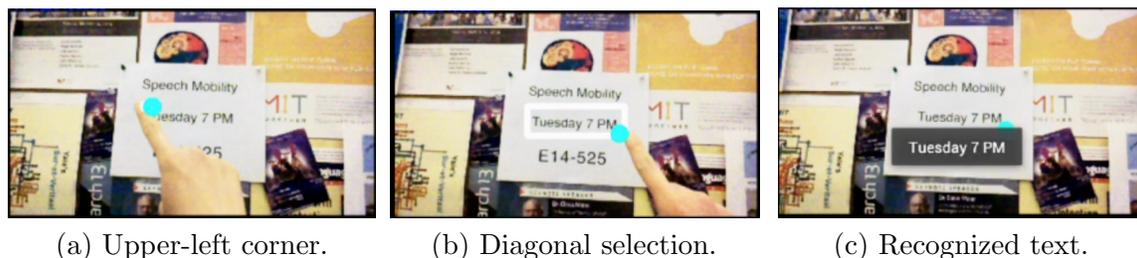
Figure 7-12: Screenshots of optical character recognition within rectangular selection implemented on Glass.
