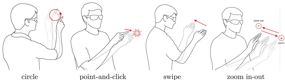
Figure 5-12: Motion-controlled gestures implemented using only the 3D coordinate data acquired by Mime’s TOF sensor.
