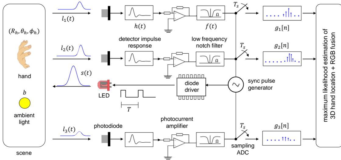
Figure 5-8: Mime data acquisition pipeline showing the system parameters and hardware components.
