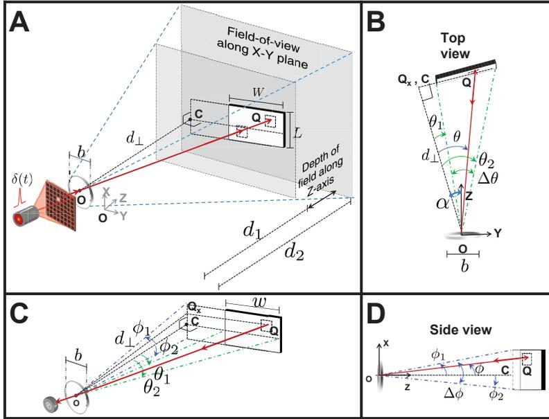
Figure 3-2: (A) Scene setup for parametric signal modeling of TOF light transport; (B) Top view; (C) Notation for various angles; (D) Side view.
