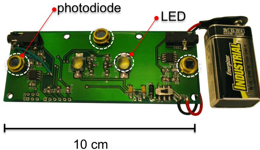
Figure 7-5: Iterated version of Mime sensor designed to map dimensions and form-factor of Google Glass and a smart phone.
