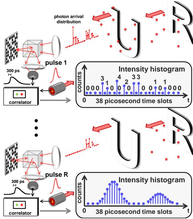
Figure 4-3: The process of generating a timing histogram. (top) For a fixed DMD pattern, scene illumination with the first pulse results in a low photon flux with a Poisson distributed photon arrival. The APD + correlator combination records the time of arrival of these photons with a 38 ps accuracy and increments the photon count in the respective time bins. (bottom) This counting process is repeated for  $R$  pulses and the entire intensity profile is generated.
