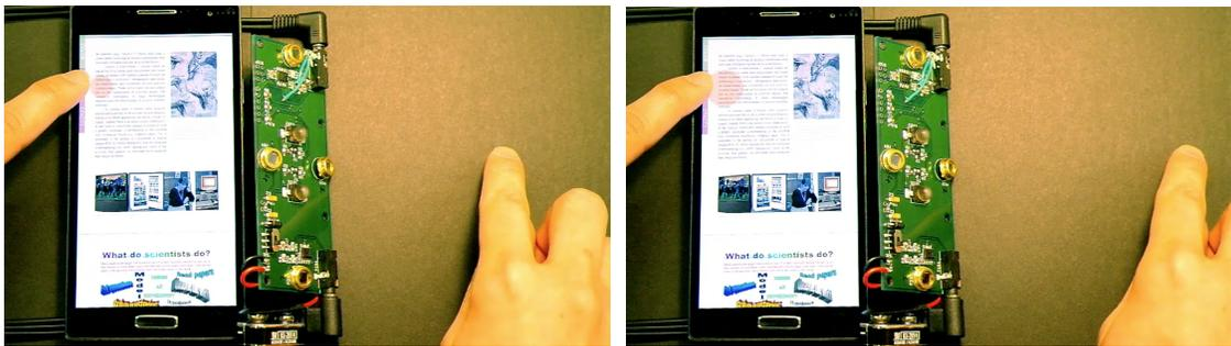
Figure 7-18: Two-handed hybrid input with touch used to select a **size** function and hand movement used to precisely control brush thickness.
