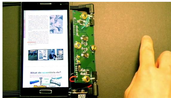
Figure 7-16: The side facing configuration of the Mime sensor is used to highlight text in a word processing task on a mobile device.
