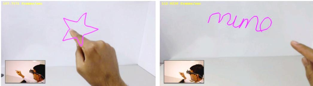
Figure 7-2: In-air writing and drawing implemented only using Mime’s TOF sensor.
