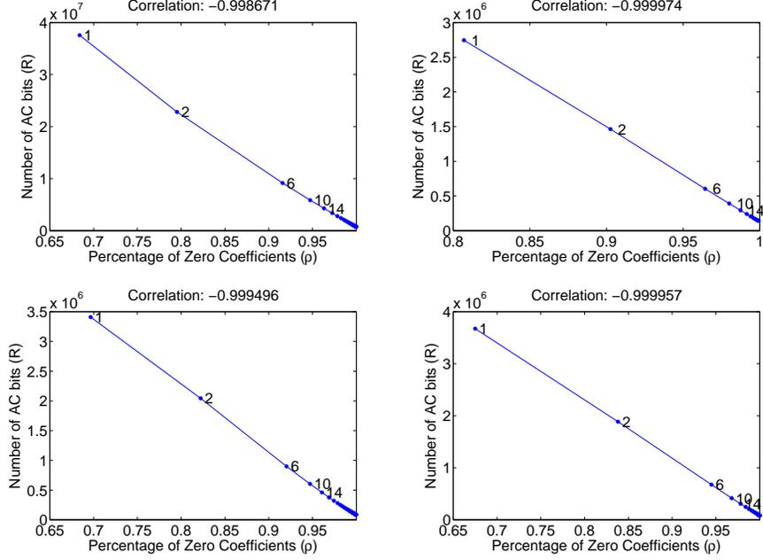
Figure 2-1: The relationship between the number of AC bits ( $R$ ) and the number of zeroes as a percentage ( $\rho$ ) of quantized AC coefficients is plotted for several images. The number next to each point indicates the scaling factor used on the quantization table of the image. Every image exhibits a correlation of nearly unity.
