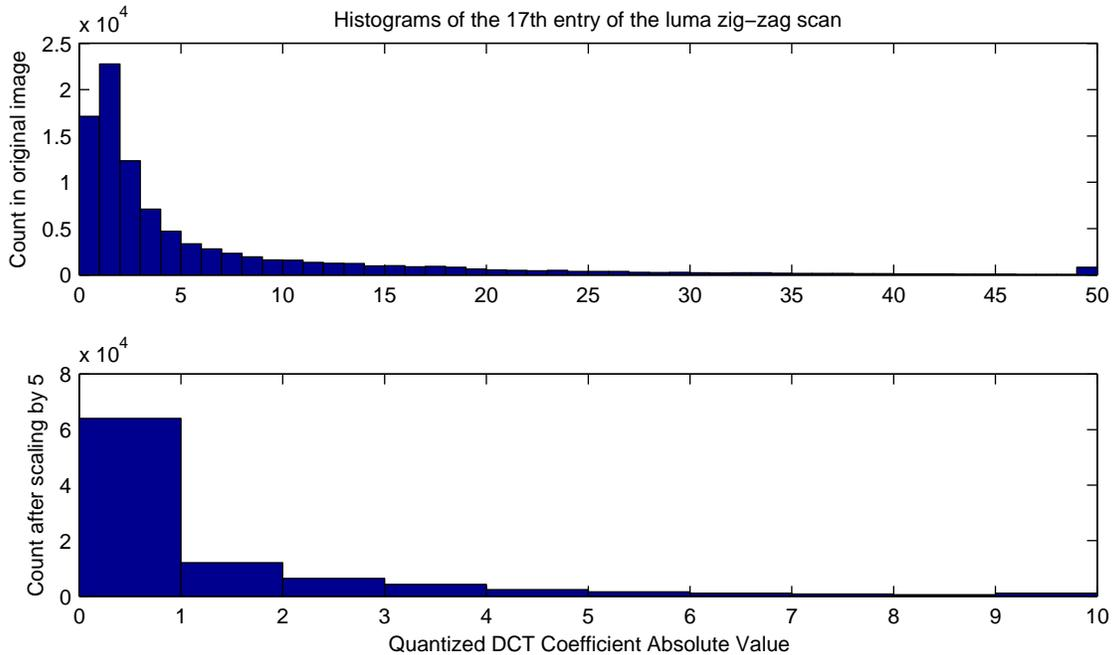
Figure 2-2: An example histogram of quantized DCT coefficients in the 17th entry of the luma
