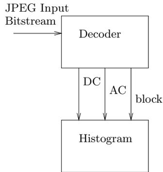
Figure 2-6: Data flow in the JPEG transcoding framework during the decoding pass (first pass). The JPEG bitstream is decoded block by block. The decoder publishes block data and DC and AC symbols to the histogram collector.
