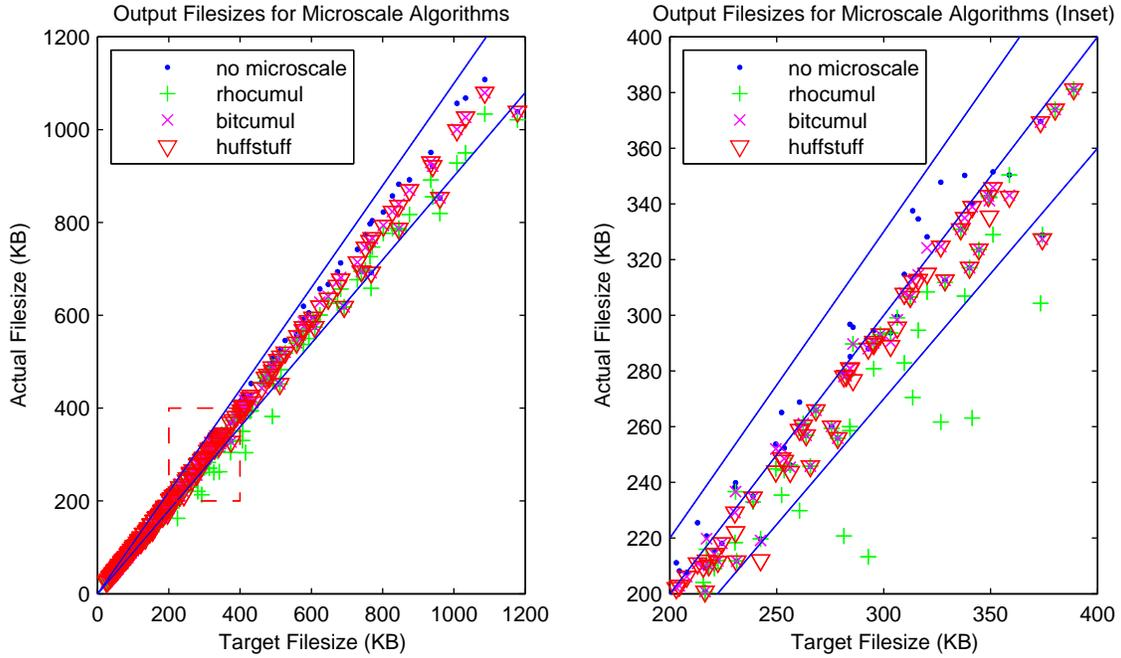
Figure 3-3: Scatter plots of output filesize vs. target filesize are shown. The  $\rho$ -cumulative algorithm tends to overcompress. The bit-cumulative and Huffman/stuff byte algorithms produce filesize errors roughly between 0% and -10%.
