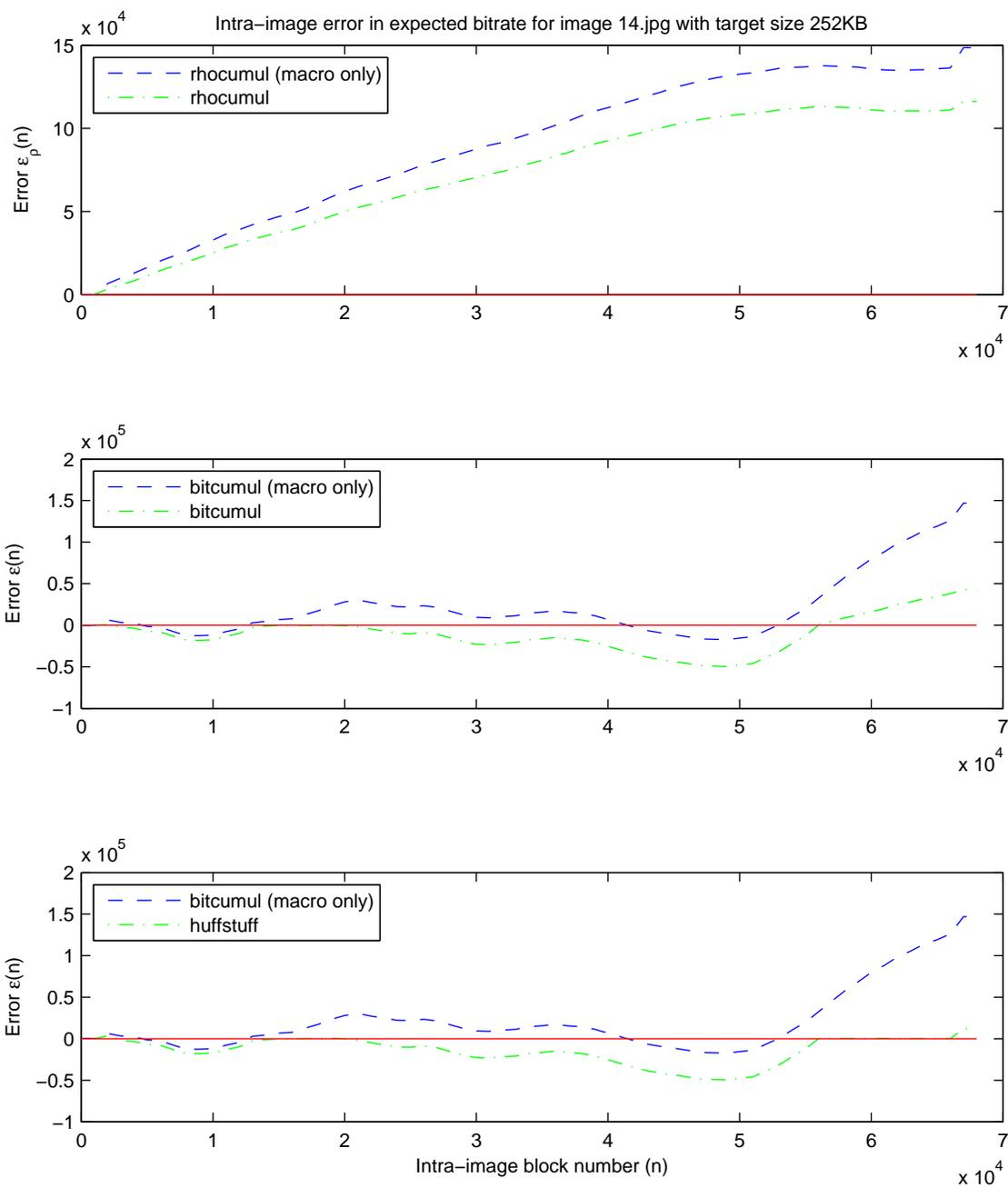
Figure 3-5: The intra-image error calculated as the difference between actual bitrate and expected bitrate. The bit-cumulative indicator produces error values near zero in the second and third plots. The Huffman/stuff byte actuator has the smallest final error in bitrate.
