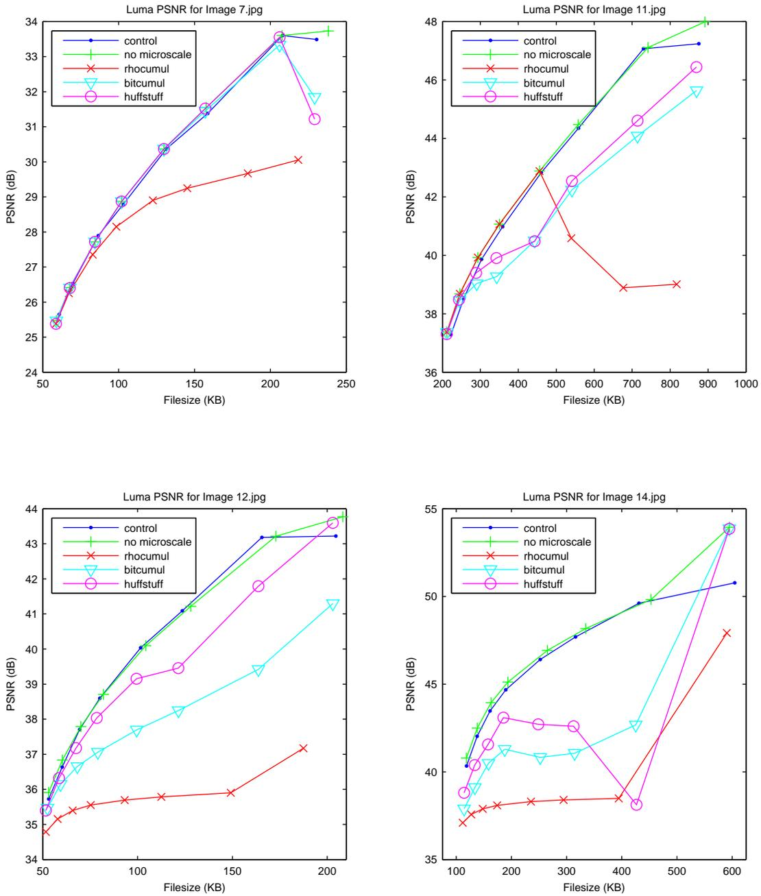
Figure 3-6: PSNR of the luma component vs. output filesize for four images using various microscale rate control algorithms. In most cases, the highest PSNR was produced without microscale control. Images from the Huffman/stuff byte algorithm usually had higher or comparable PSNR to images from the bit-cumulative algorithm. The  $\rho$ -cumulative algorithm consistently produced the lowest PSNR.
