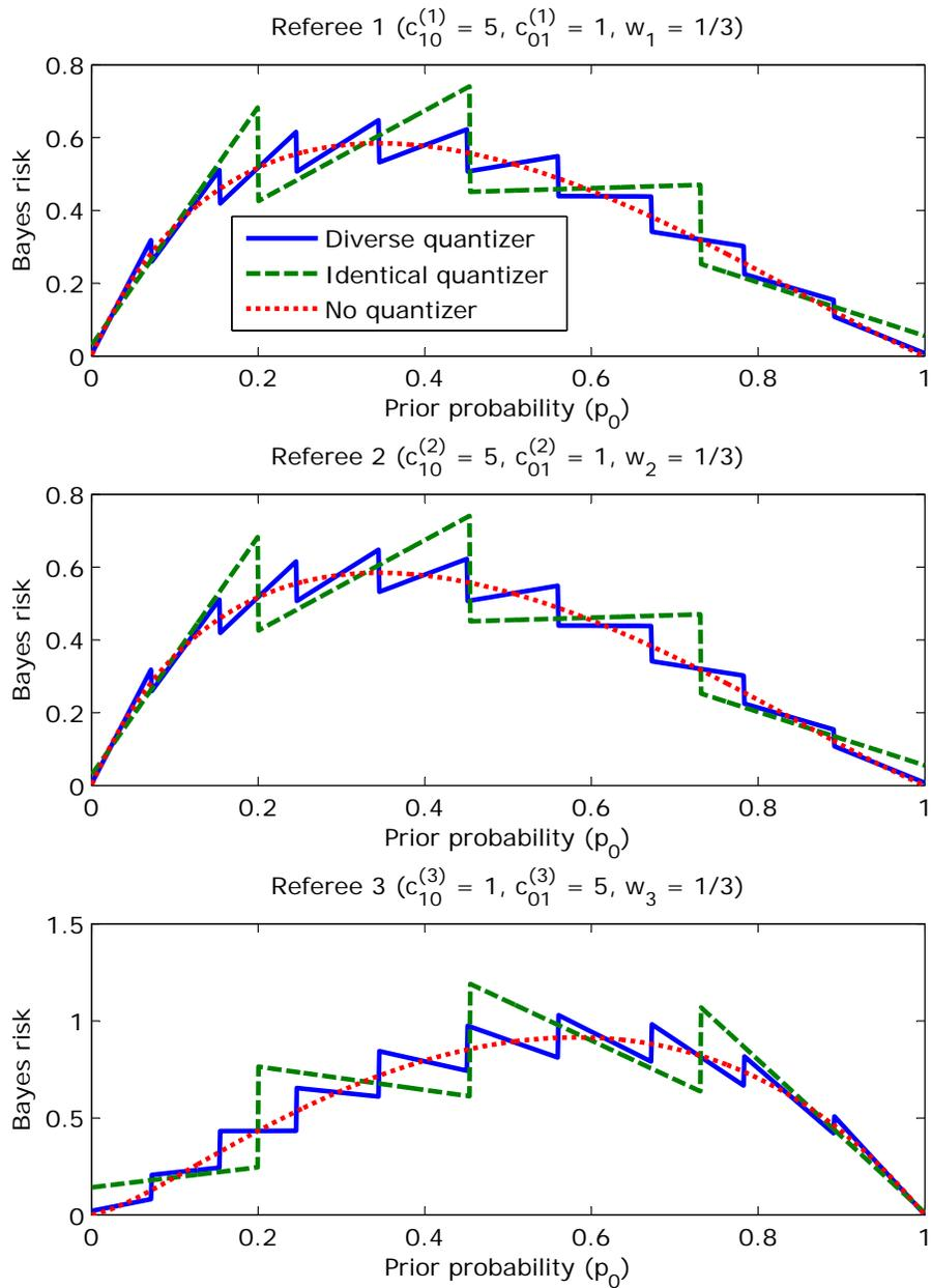
**Figure 4-12.** Quantizers for uniformly distributed  $P_0$ ,  $h_0 = 0$ ,  $h_1 = 1$ ,  $\sigma = 1$ , and non-identical referees.
