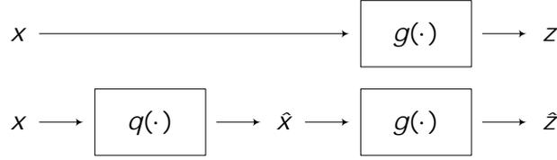
**Figure 2-2.** Fixed-rate scalar functional quantization.
