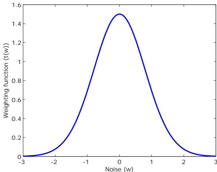
**Figure 3-4.** Weighting function  $t(w)$  for the realization of noise  $W$ , which has the Gaussian density of  $\mathcal{N}(0, 1)$ .
