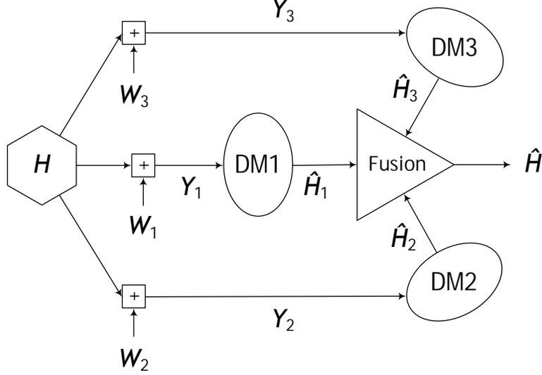
**Figure 3-1.** The distributed detection and fusion model explored in this work.
