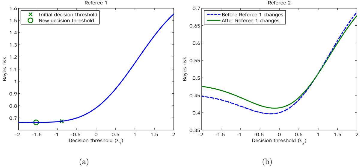
**Figure 4-2.** Change of the Bayes risks that shows how referees conflict. Referee 1 has Bayes costs  $c_{10}^{(1)} = 1$  and  $c_{01}^{(1)} = 4$ , referee 2 has  $c_{10}^{(2)} = 4$  and  $c_{01}^{(2)} = 1$ , and referee 3 has  $c_{10}^{(3)} = 4$  and  $c_{01}^{(3)} = 4$ .  $p_0 = 0.5$ . (a) The Bayes risk of Referee 1 for his decision threshold. (b) The Bayes risks of Referee 2 before and after Referee 1 changes his decision threshold.
