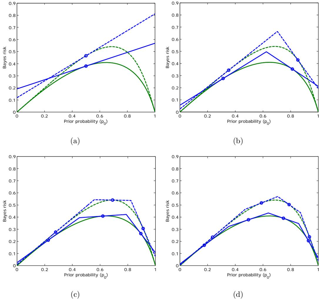
**Figure 3-8.** Quantizers for uniformly distributed  $P_0$ ,  $h_0 = 0$ ,  $h_1 = 1$ ,  $\sigma = 1$ , and Bayes costs  $c_{10} = 1$  and  $c_{01} = 4$ . Mismatched Bayes risk and unquantized Bayes risk are plotted for (a)  $K = 1$ , (b)  $K = 2$ , (c)  $K = 3$ , and (d)  $K = 4$  in three-referee model (as solid line) and single-referee model (as dashed line).
