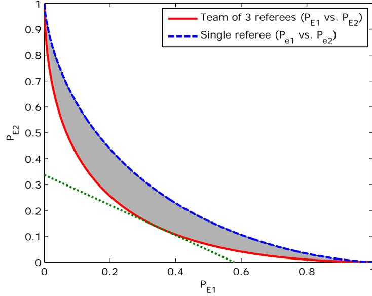
**Figure 3-2.** The operating region of the three-referee model for  $h_0 = 0$ ,  $h_1 = 1$ , and  $\sigma = 1$ . The green dotted line depicts (3.7) for  $c_{10} = 1$ ,  $c_{01} = 4$ , and  $p_0 = 0.7$ .
