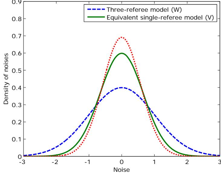
**Figure 3-5.** The density of noise  $V$  in a single-referee model that is equivalent to the three-referee model with noise  $W$ , which has the Gaussian density of  $\mathcal{N}(0,1)$ . For comparison, the density of  $\frac{1}{3}W$ , the effective noise of soft decision-making referees, is drawn in red dotted curve.
